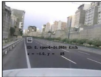
Figure.5 Detected car coming with determining speed
